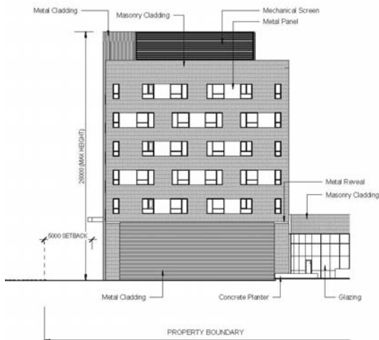
⊕ WEST ELEVATION NORTHWEST TOWER
