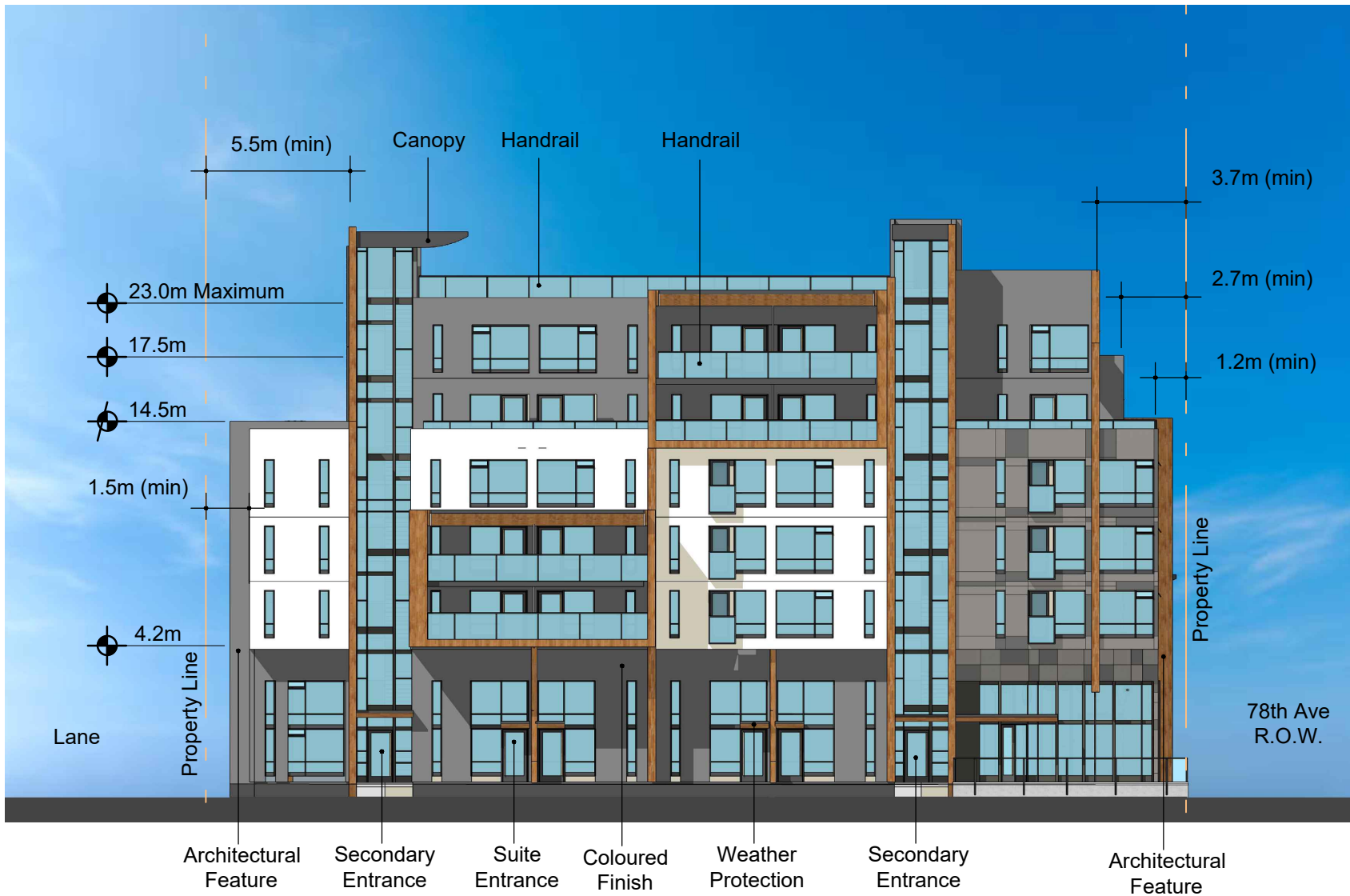
APPENDIX 8a (South Building) - EAST ELEVATION
