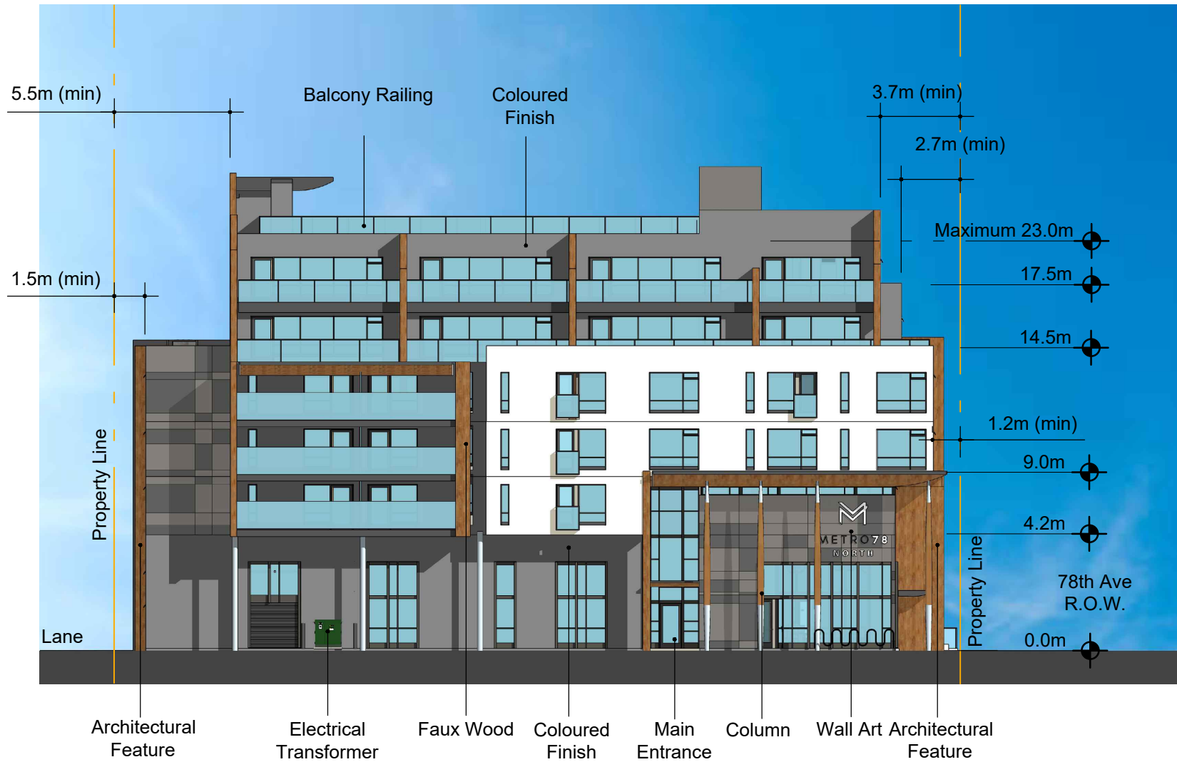
APPENDIX 7b (North Building) - WEST ELEVATION
